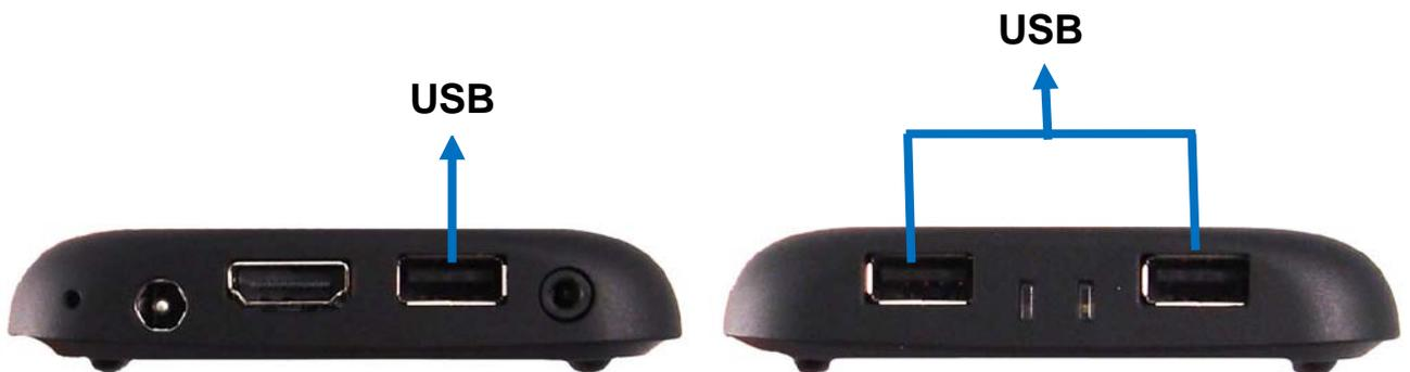
*Figure 4 Connect USB mouse & keyboard*
