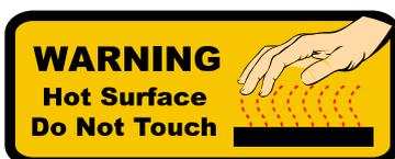
The product chassis may be hot when the system is working. Please do not touch the surface before turn off the system power and wait for about 5 minutes until the system cools down.
