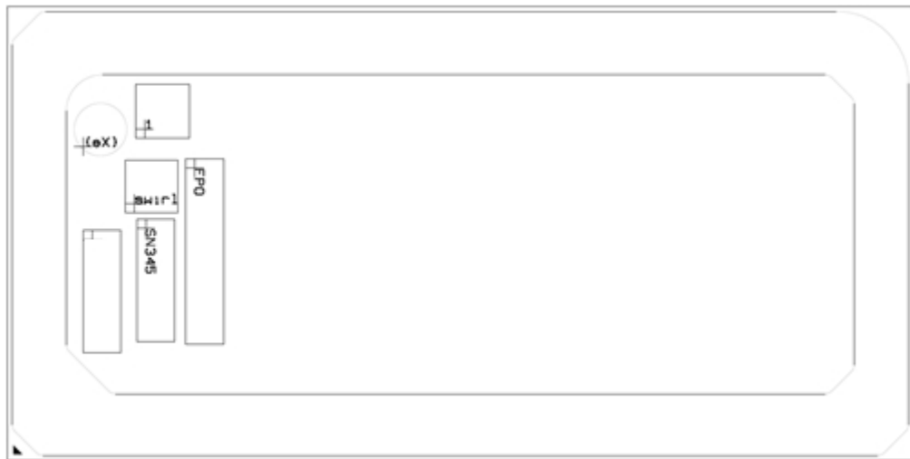
Figure 2-3. Processor Based on U15 Processor Line Chip Package BGA Top-Side Markings
