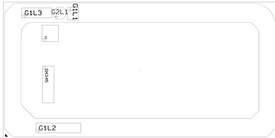
Figure 2-2. Processor Based on H/P-Processor Line Chip Package LGA Top-Side Markings
