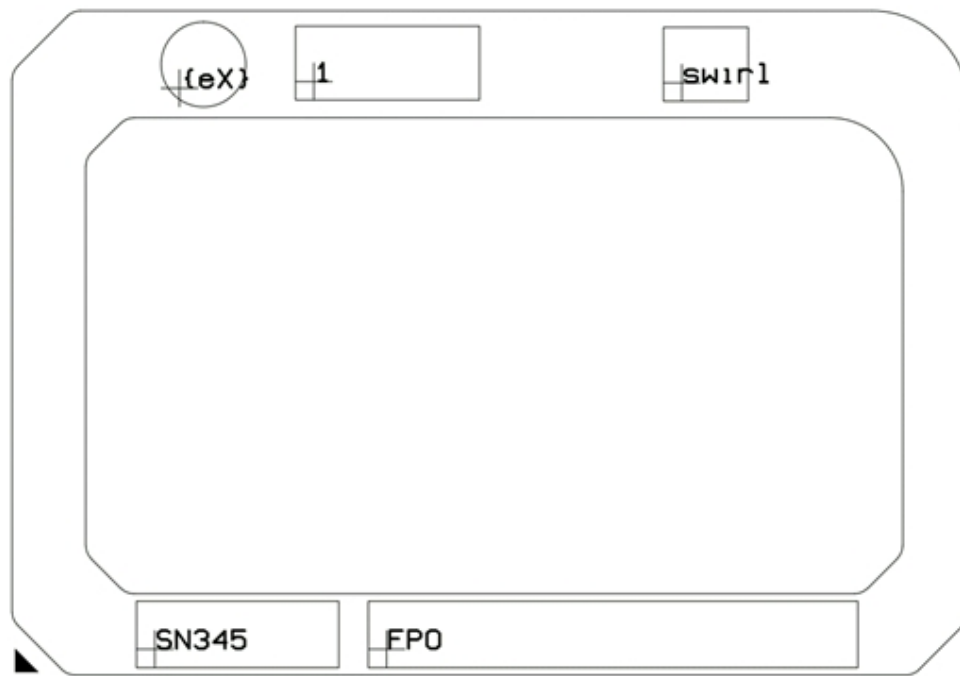
Figure 2-2. Processor Based on UP4 Processor Line Multi-Chip Package BGA Top-Side Markings
