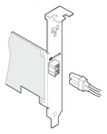
Most connectors and ports are keyed for proper orientation. If the cable you are using is not keyed, check to be sure the connector is oriented properly (transmit port connected to receive port on the link partner, and vice versa).
