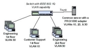
Typically, VLANs consist of co-workers within the same department but in different locations, groups of users running the same network protocol, or a cross-functional team working on a joint project.
