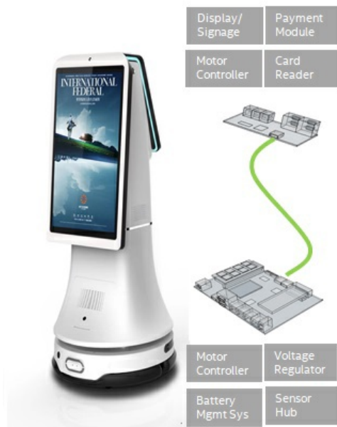
Figure 2 A typical service robot structure
