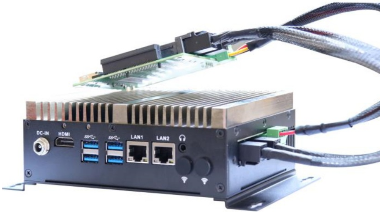
Figure 5 shows the mini SAS interconnection between the main compute board and I/O expansion board.
