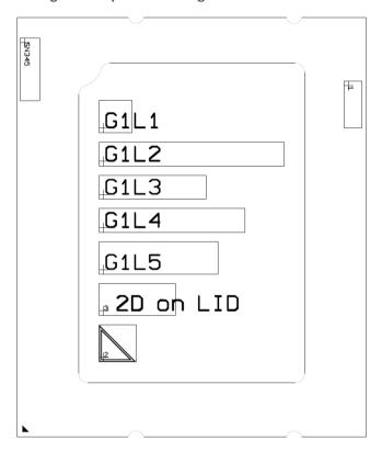
Pin Count: 1700 Package Size (width x height): 37.5mm x 45mm
